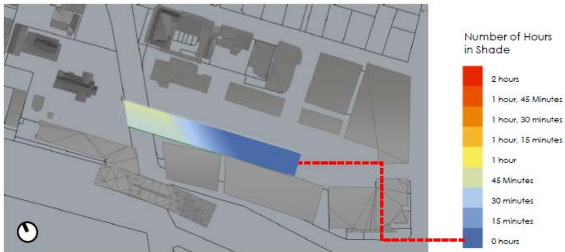
Extract from *Inhabit Report* at Appendix 13 showing average duration of overshadowing of a single point in the DCP solar zone is less than 19 minutes
